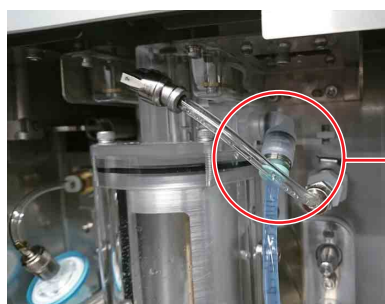
Coupling points toward the front, blocking the door.
