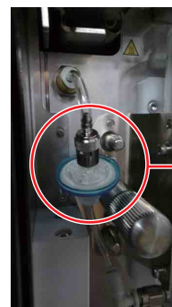
Push air filter toward the rear to clear the door.
