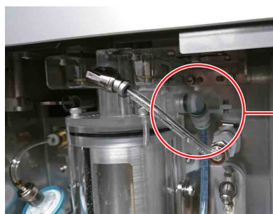
Push coupling toward the rear so tubes clear the door.
