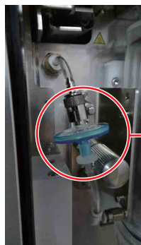
Air filter protrudes at the front, blocking the door.
