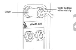
The waste tank can become pressurized when the cytometer is running. Always disconnect the tank from the fluidics cart before you empty it. Wait at least 30 seconds for pressure to dissipate before you remove the waste cap or level sensor cap.
