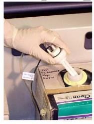
Put a new container onto the fluidics cart.
