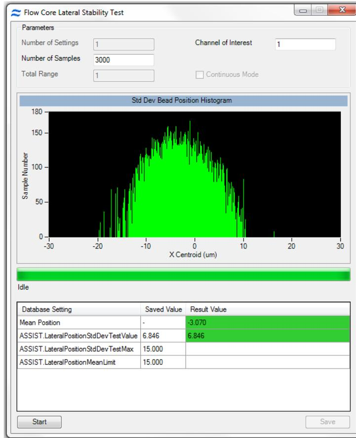
Contaminated sheath, obstructions, air or improper pump function may broaden the core which can reduce focus consistency and increase variation in intensity measurements. This flow core lateral stability ensures the core is operating as designed with minimal variation. Failure to pass this test is indicative of at least one of the issues listed above.
