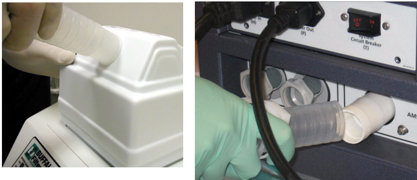
Figure C-10 Connecting new tubing
