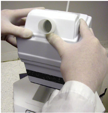
Figure C-8 Inserting the new filter
