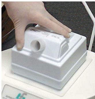
Figure C-9 Seating the new filter
