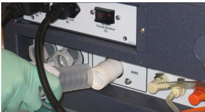
Figure C-6 Disconnecting tubing (side of instrument)
