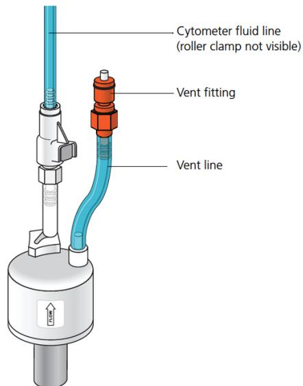
➤ **Check the sheath line for air bubbles.**
